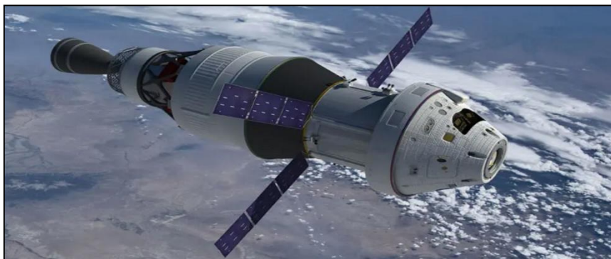
Left: The configuration with solar panels deployed, before Trans-Lunar Injection (TLI), after which the left-hand half of the vehicle (the ICPS) separates and is lost. The right-hand half (the Orion) heads to the Moon. Right: The three sections of the Orion spacecraft, showing two ICPS/Orion interstage panels detached.
