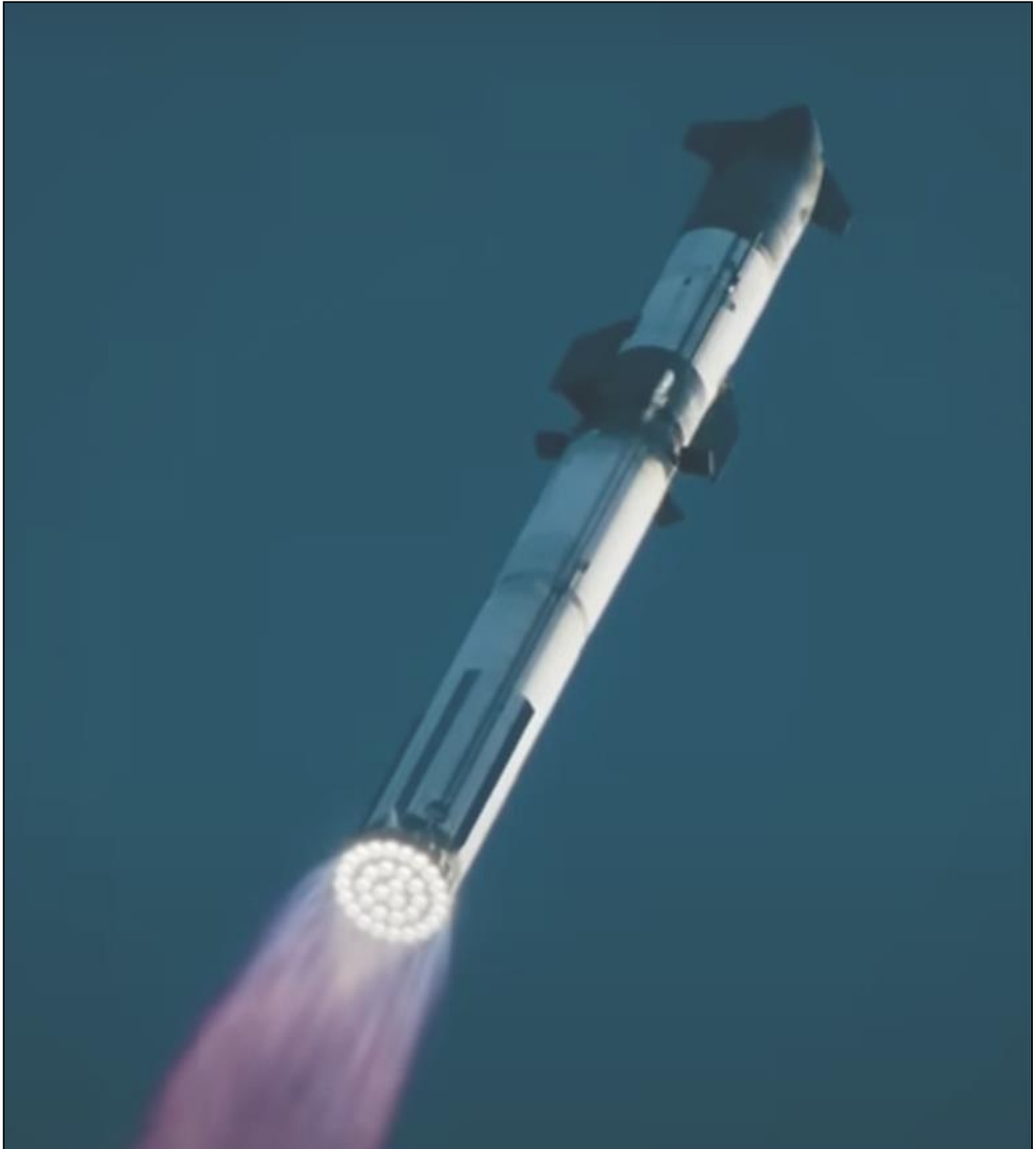
SpaceX's Super Heavy Booster 9 + Starship 25 lifts off from Starbase in southern Texas, soon after 8 am local time on 18 November 2023, with all 33 Raptor engines firing. See pages 16-17 for a report on the flight.
